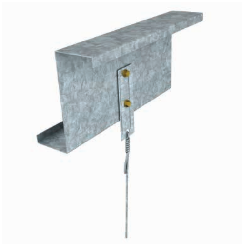
■ FIGURE B2.4.4(G): 2.5mm WIRE ATTACH TO 274 BRACKET WITH 3 FULL TIGHT TURNS
