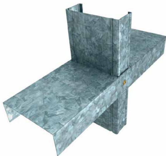
■ FIGURE C2.4.5(G) NOGGING FIXING DETAILS
