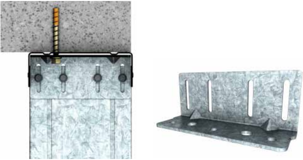
■ FIGURE C1.7.4(A): SLOTTED BRACKETS
