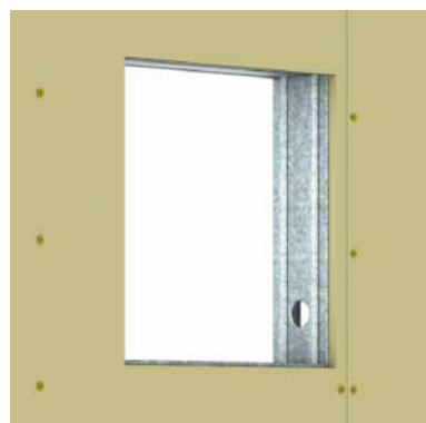
■ FIGURE E1.4.3.1(D): CONSTRUCT SUPPORTING STRUCTURE
